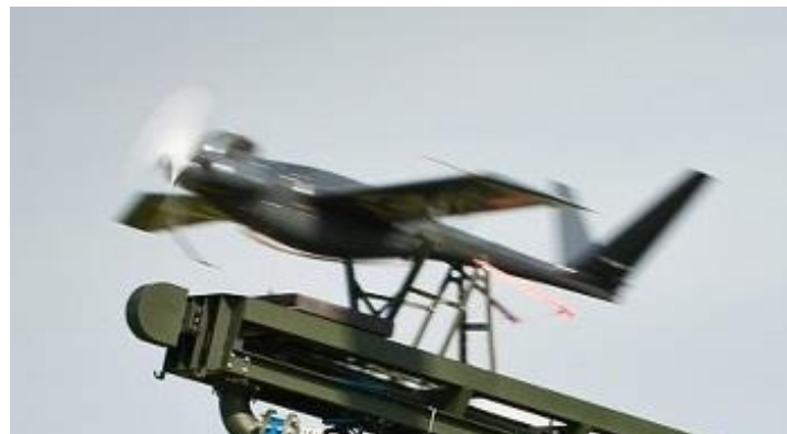
Fig. 1 – Small UAV launch from an air-powered catapult
